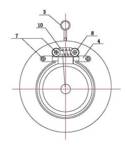
Working Pressure : 4.0 Mpa Seal Pressure Test : 4.4 Mpa Body Pressure Test : 6.00 Mpa Valve Design : ASME B16.34
