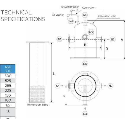
**Design Pressure:** 5 bar **Design Temperature:** 198°C
