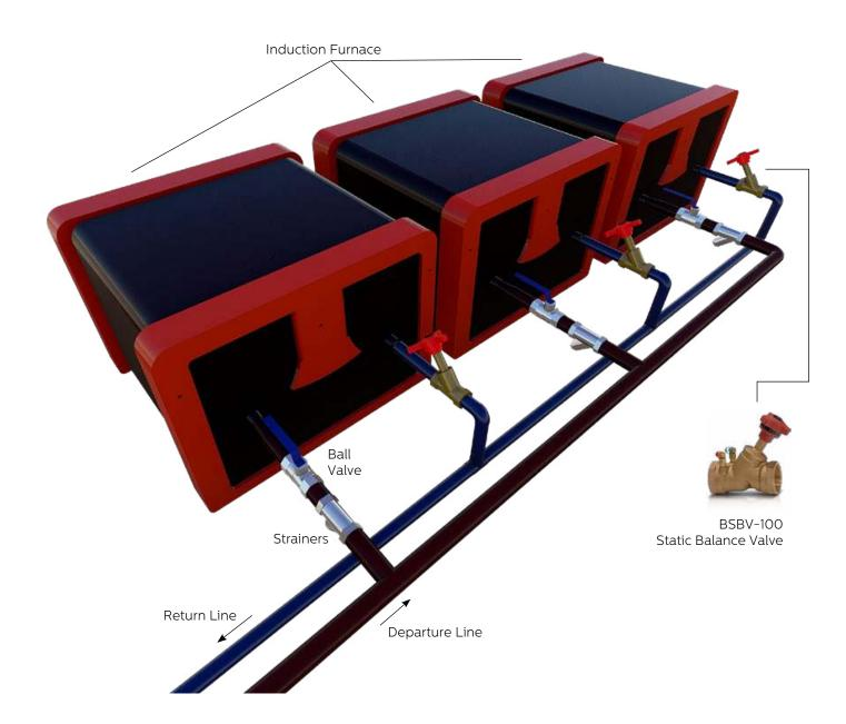
**Note:** It prevents the flow above the required cycle for heat transfer and ensures a more reliable, balanced and healthy operation of the system. It can be adjusted manually by the manuel adjustable throttle disc on it.
