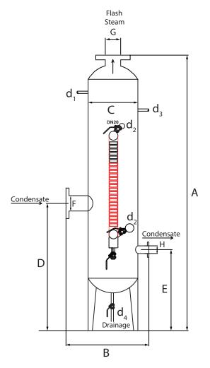
Note: The maximum value of the amount of flash steam generated corresponding to the maximum condensate amount is as follows, which is the result of highest pressure (14-15 bar) move into the atmospheric pressure 0 bar.
